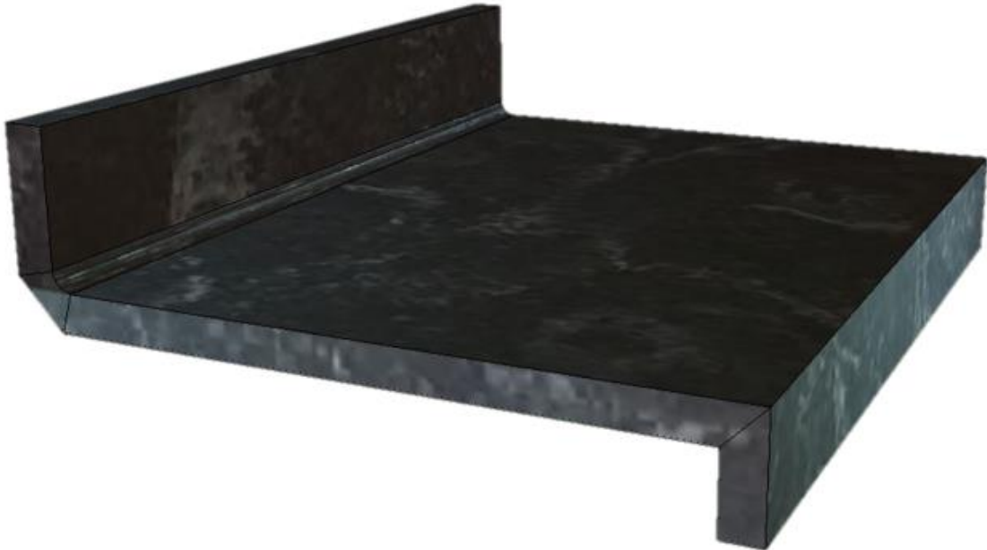
Figure 20. V-groove technique folded together
