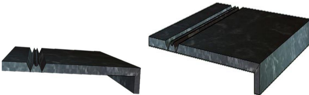
Figure 21. V-Groove edge before gluing and folding
