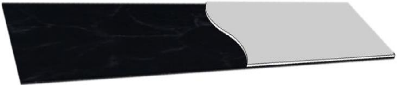
Figure 6. Template used to cut serpentine seam
